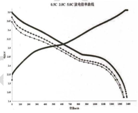
0.5C 0.0C 5.0C Discharge rate curve
