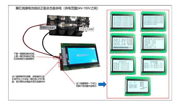
On/off switch, use GND and SW signal.
