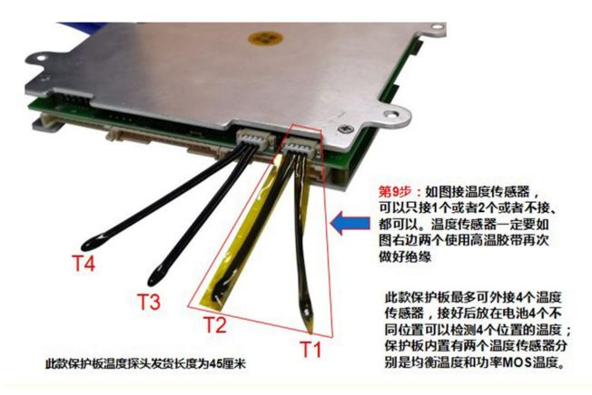
It is recommended to wrap the NTC with high temperature insulating glue for good insulation
