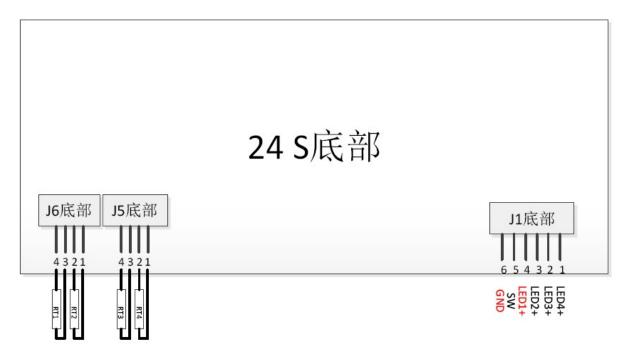
J5 and J6 for temperature sensor J1 for switch ( on/ off switch), use GND and SW signal.
